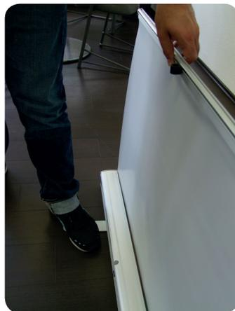
6. Clamp the rod at the top first. Then use the rod to push the print fully up.
